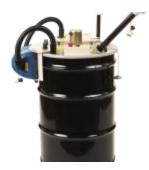
Properly dispose of this material to prevent its exposure to the environment. With the assistance of our new bulb eater from Air Cycle Corporation, we can crush mercury containing fluorescent tubes and CFL Bulbs. Keep Carroll Beautiful will dispose of the bulbs under governmental EPA standards. We accept all lengths of fluorescent bulbs, as well as, round and U-shaped fluorescent bulbs.
